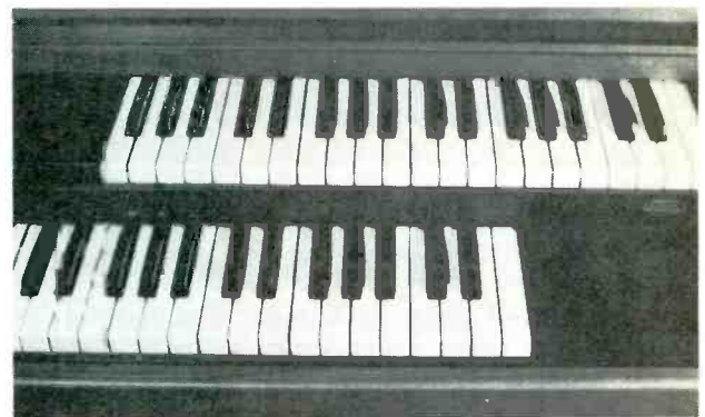
Fig. 5 The solo (swell) keyboard usually is played by the right hand, so the lower notes are eliminated to minimize the cost. In the same way, the higher octave of the accompaniment (great) keyboard is not provided. However, the notes of the two keyboards match, C above C, G above G, etc.
